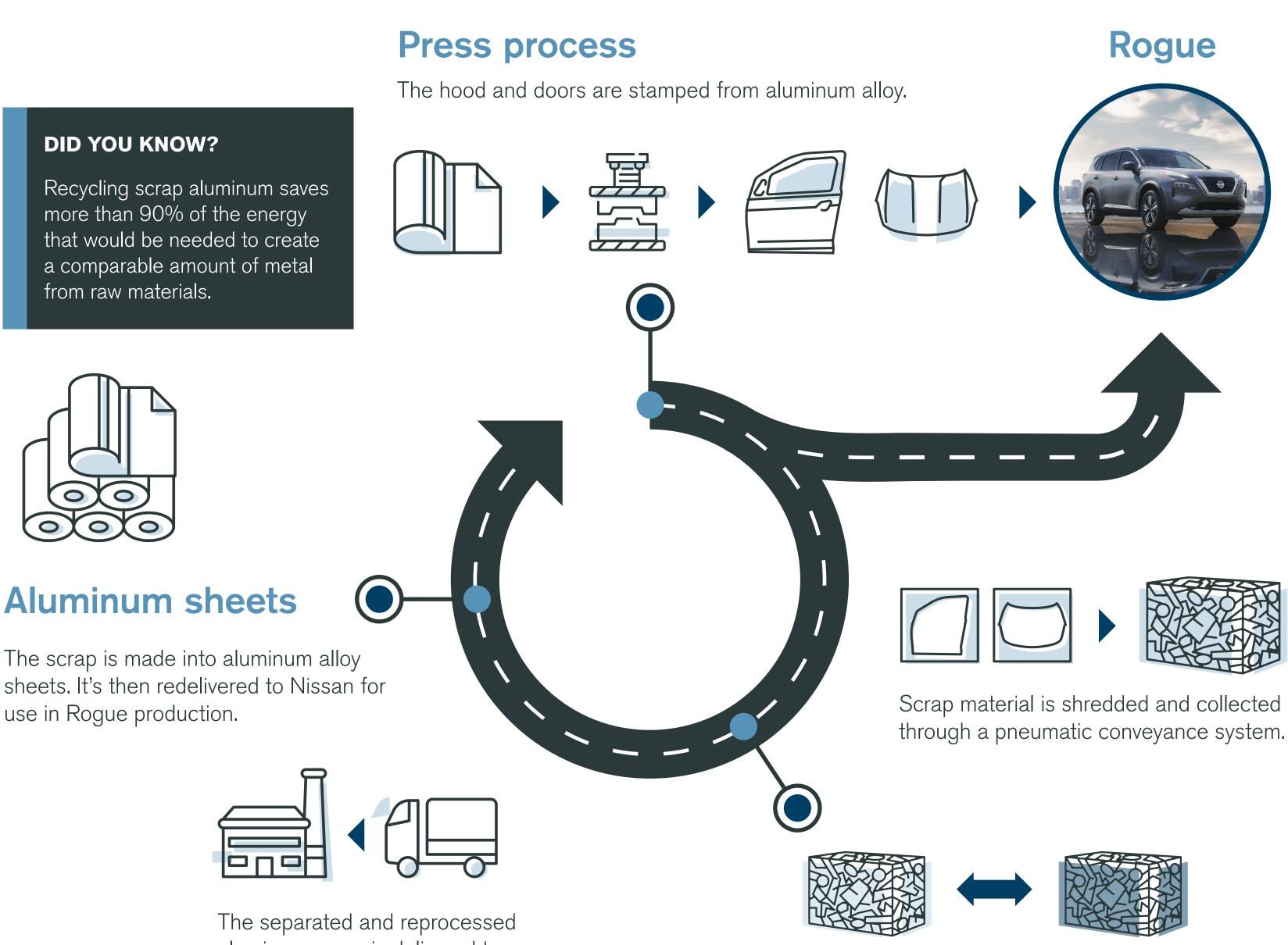
The separated and reprocessed aluminum scrap is delivered to the aluminum supplier.
