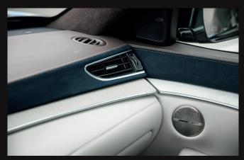
Using bespoke manufacturing methods, 'wrap and sew' detailing is a highlight of the hand-crafted ambience. The leather on the dash is selected for its quality and is hand-wrapped over panels
