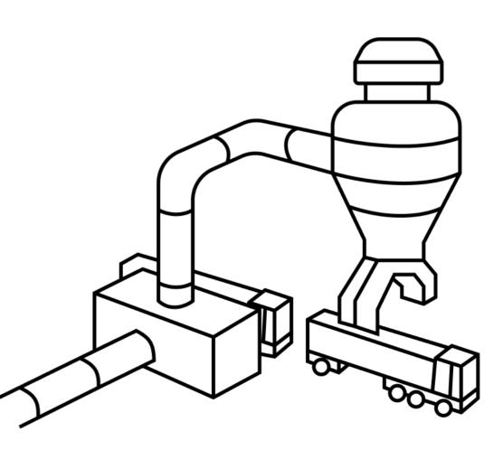
Reprocessed scrap is delivered to the aluminium supplier for recycling
